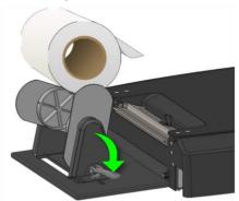
d Insert stock into input slot
