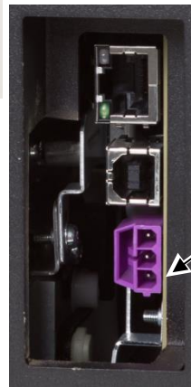
Connect the Power Supply to the Printer
