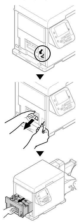
19 While supporting the fuser and exit unit with one hand, lift up the fuser and exit unit handle.
