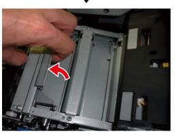
12 While the paper guide release lever is lifted, slide the paper guide in the direction of the arrow to remove it.
