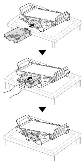
13 When facing the belt unit, hold the handles (blue) on its left and right sides.
