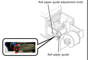
16 If there are scraps of paper or glue from labels on the ends of the sheet guide, undo the screw and remove the unwinder paper guide.
