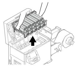
10 Place the removed print cartridge, and cover it with paper so it is not exposed to light.
