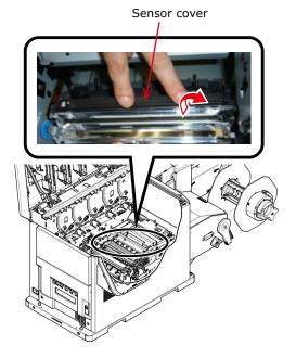
17 Use Wiper moistened with cleaning fluid (anhydrous) to wipe, in one direction, the dirt off the sensor cover (lower and upper).
