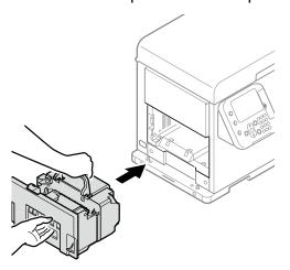
Push down the fuser and exit unit handle, and firmly push it inside.
