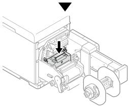
(2) Lower the cutter unit lock levers at both ends of the cutter unit.
