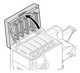
2 Check the position of the print cartridge to replace, by the text and color of the label.
