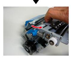
Slide the F1 roller unit at an angle (arrow direction) and remove it.
