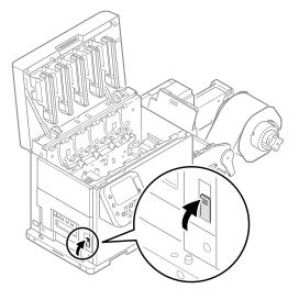
Confirm that the blue levers in the unwinder are raised, and then remove the cutter unit.
