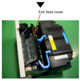
23 Slowly pull out the paper that is left in the fuser and exit unit in the direction of the arrow.
