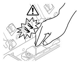
13 Hold the belt unit handles (blue) on the left and right, and remove the belt unit at an angle.
