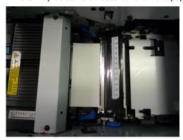
Be careful, the fuser and exit unit is very hot immediately after printing. 17 If paper is being output from the printer, use scissors to cut it between two labels.
