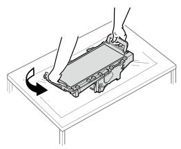
14 Tilt the belt unit and align the arrow labels (red) on the belt unit and printer to position it, and then open the belt unit handles (blue) on the left and right.
