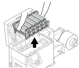
Place the removed print cartridge, and cover it with paper so it is not exposed to light.
