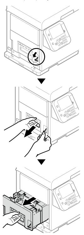
While supporting the fuser and exit unit with one hand, lift up the fuser and exit unit handle.
