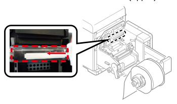
Use Wiper moistened with cleaning fluid (anhydrous) to wipe, in one direction, the dirt off the sensor cover (lower).
