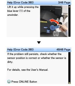
Removing the jammed paper will return the display to the Standby screen and the remaining printing will start.
