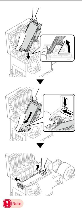
Be careful to not pinch your hands or fingers between the handle and the machine while installing the belt unit. Turn the two belt locking keys clockwise to lock it.
