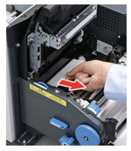
**31** Raise the blue lever and install the cutter unit.
