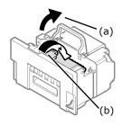
25 Lift the fuser and exit unit with both hands and put it into the printer.
