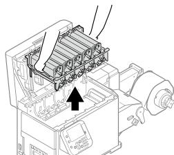
Place the removed print cartridge, and cover it with paper so it is not exposed to light.
