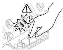
15 If the rollers and feed surface of the feed unit on the bottom of the paper guide are dirty, gently wipe them clean with Wiper or cleaning sticks moistened with cleaning fluid (anhydrous).
