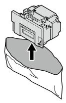
Pull the fuser and exit unit locking lever on the new fuser and exit unit towards yourself, and lift the fuser and exit unit handle.
