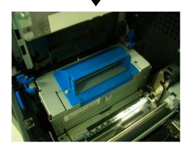
32 Align the positions of the paper guide's edge ( ① ) and the guide notch on the printer.
