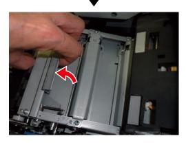
16 While the paper guide release lever is lifted, slide the paper guide in the direction of the arrow to remove it.
