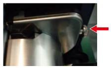
19 Turn the screws in two locations on the F0 roller unit to loosen them.
