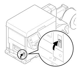
Align the positions of the paper guide's edge ( 1) and the guide notch on the printer.
