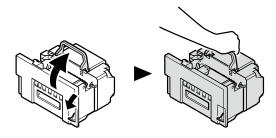
Lift the new fuser and exit unit with both hands and put it into the printer.
