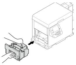
25 Push down the fuser and exit unit handle, and firmly push it inside.
