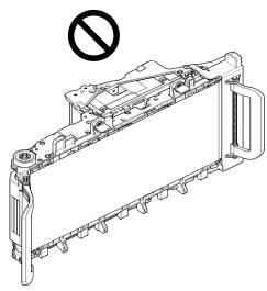
• Do not touch the belt surface or damage the belt.
