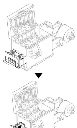
Hold the fuser and exit unit with both hands and remove it to a level spot.
