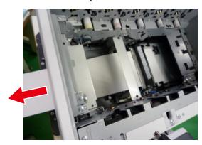
22 Lower the release lever of the fuser and exit unit, open the exit feed cover and put the fuser and exit unit handle below the exit feed cover.
