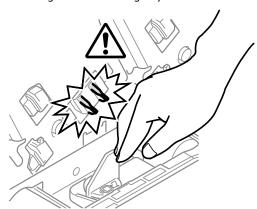
**17** Put the print cartridge set back into the printer.
