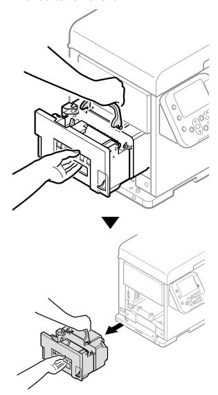
Remove the new fuser and exit unit from its packaging.
