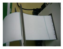
18 While pulling the fuser and exit unit locking lever towards you, pull out the fuser and exit unit.
