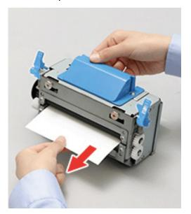
30 Remove any paper that is left in the paper feed path in the unwinder.
