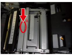
Tilt the belt unit and align the arrow labels (red) on the belt unit and printer to position it, and then open the belt unit handles (blue) on the left and right.
