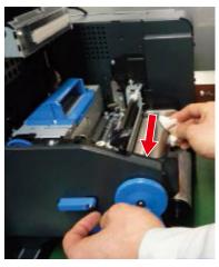
Move the roll paper guide to confirm that there is no glue or paper scraps on it. If there are scraps of paper or glue from the labels on it, use Wiper moistened with cleaning fluid (anhydrous) to wipe it off.
