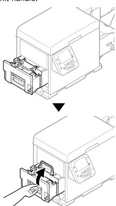
Hold the fuser and exit unit with both hands and remove it to a level spot.
