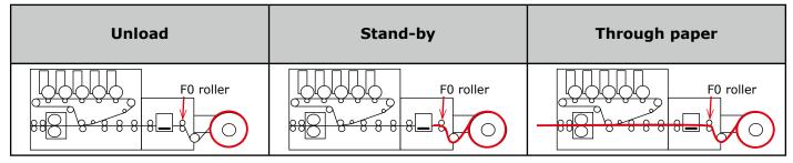
Unload: Indicates that the paper is not set on the F0 roller on the unwinder.
