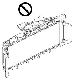
• Do not touch the belt surface or damage the belt.
