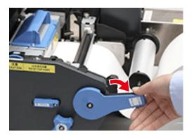
12 Lower the unwinder cover open lever to open the unwinder cover.
