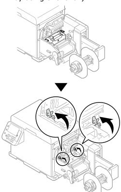
(3) Hold the handle of the cutter to remove the cutter unit.
