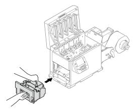
Push down the fuser and exit unit handle, and firmly push it inside.
