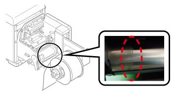
Use Wiper moistened with cleaning fluid (anhydrous) to wipe, in one direction, the dirt off the sheet guide.
