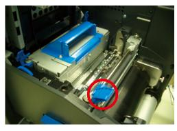
Lower the cutter unit lock levers at both ends of the cutter unit.
