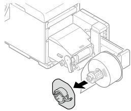
Turn the roll paper holder knob in the direction of the arrow to narrow the shaft of the roll paper holder.
