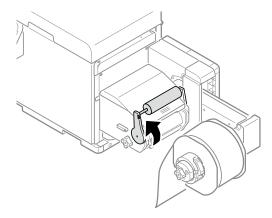
While restraining the tension bar with one hand, use Wiper moistened with cleaning fluid (anhydrous) to wipe, in one direction, the dirt off the tension bar (1).
