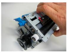
Slide the F1 roller unit in the direction of the arrow.
