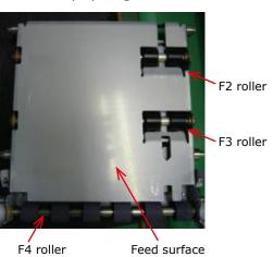
Use Wiper moistened with cleaning fluid (anhydrous) to wipe the dirt off the F4 roller, F3 roller, F2 roller, and feed surface of the paper guide.
