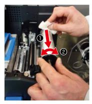
Use the hand that is restraining the tension bar to rotate it (②) as you finish cleaning each side, until the entire tension bar is clean.
