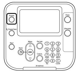
"Shutting down. Please wait. Printer will turn off automatically." appears on the control panel and the LED lamp on the <POWER> button flashes at one second intervals.
