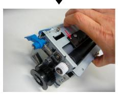
Slide the F1 roller unit in the direction of the arrow.
