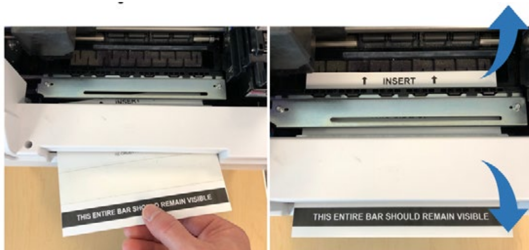
3. Unload label stock from the printer. Insert the cleaning card into the front output of the printer.
