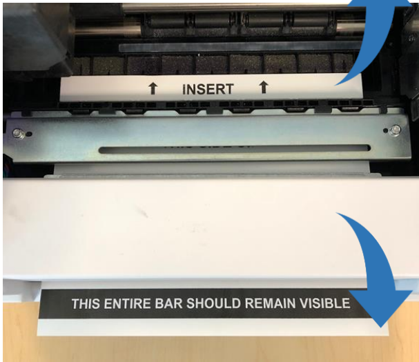
4. When the exposed adhesive strip is aligned with the output cutter path, open PrintHub – Select Printer Settings – Advanced. Click on Output Cutter Cleaning. Once the cutter cycles, remove both parts of the card from the printer.
