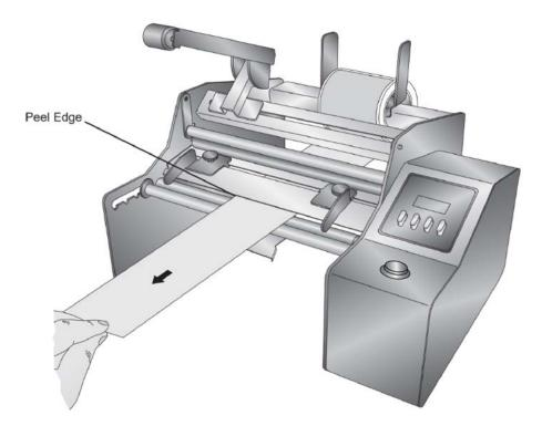
9. Take the loose label stock and feed it between the liner idler roller and the liner drive roller. In order to feed the label stock between the rollers, the liner idler roller should be in the unclamped position.
