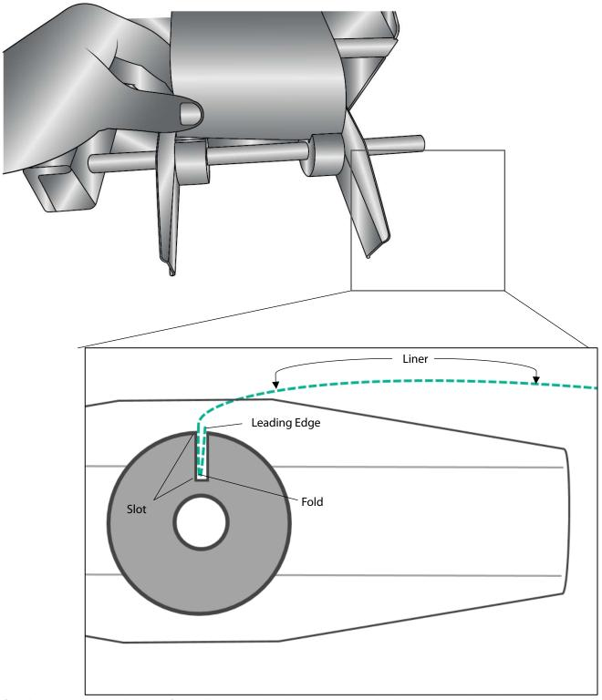
**Tip:** If the liner is slippery and doesn't fold well or stay in the slot, you can tape the liner to the guides to keep it in place. Use low tack tape that has a long cure period such as blue painters tape. You may also use the applicator without using the liner rewinder by removing the liner guides and letting the linder fall over the shaft onto the floor.
