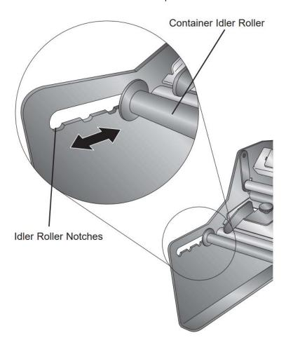
3. Place the container on the container idler roller and container drive roller. Orient the container with the top to the left or the right, depending on the orientation of your labels on the label stock roll.
