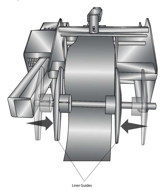
15. Fold the leading edge of the liner so the folded edge is in the bottom of the slots on both liner guides. **Tip!** We recommend cutting the liner shorter so that you have as little slack as possible between the liner clamp and the rewinder as possible. It will also give you a nice clean edge to fold.
