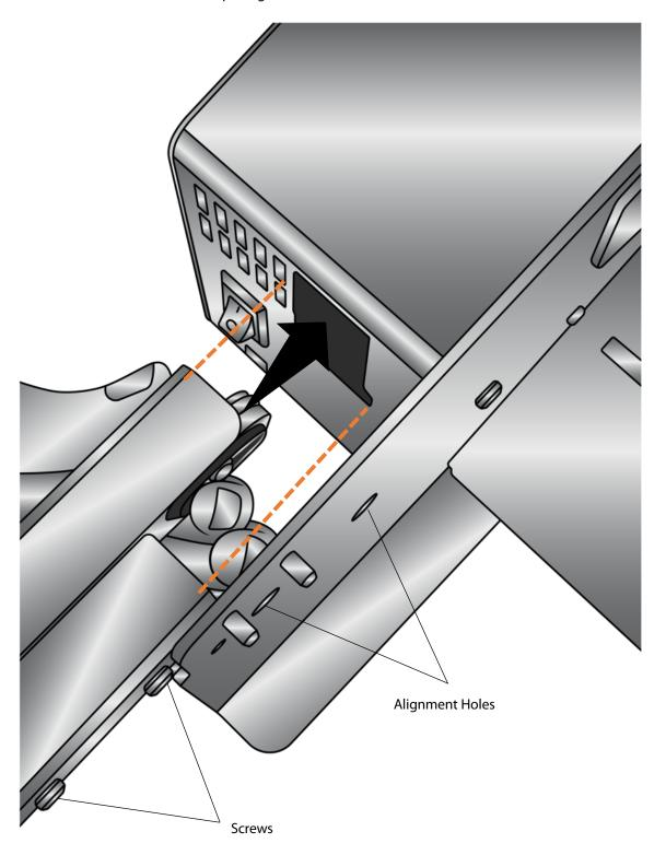
4. Align the screws on the side of the arm with the holes in the applicator frame.
