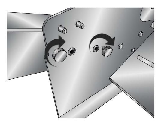
6. If not already attached to th rewinder arm, the liner guides must be installed on the rewinder. Locate the liner guides. Slide one of the label guides onto the shaft with the black cylinder facing you. Note that the holes in the cylinder must align with the flats on the shaft.
