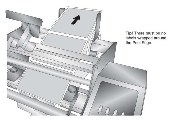
11. If necessary, adjust the position of the liner on the peel edge left/right to align the liner with the label stock roll. Also, adjust the label sensor using the label sensor bracket so that the label sensor flag is roughly centered on the label stock.
