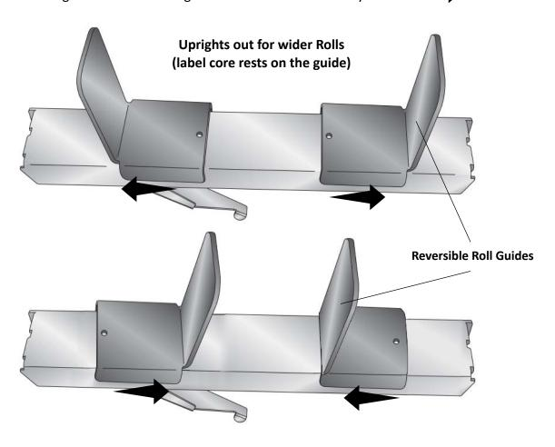
Uprights in for narrow Rolls (label core rests on the bar)
