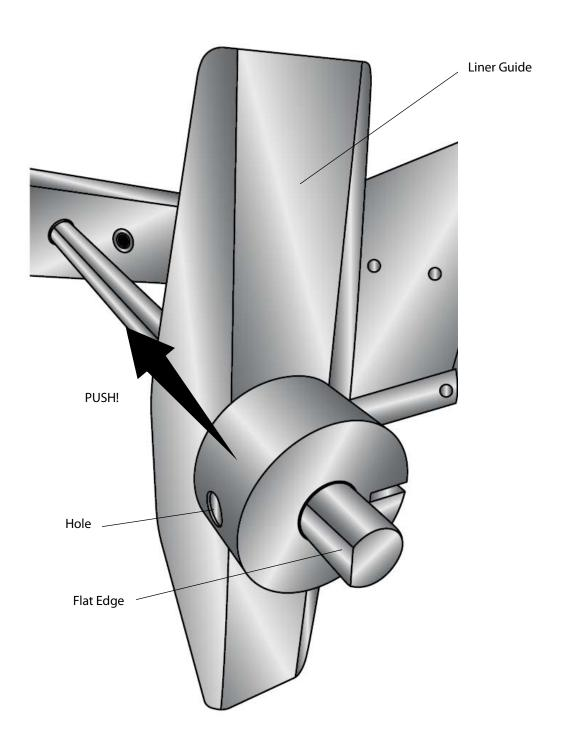
7. Push the remaining liner guide onto the shaft with the black cylinder facing away from you. The guides should be calibrated from the factory to stay in place during label application, but allow adjustment of their position without the use of tools. If more or less sliding force is desired, the set screws in the black cylinders can be tightened or loosened with a 2mm hex key. The two set screws in each cylinder should be tightened equally.
