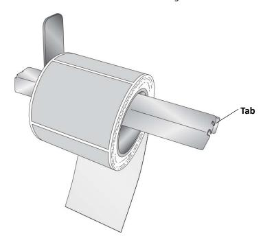
**Tip!** For smaller width label roll cores (less than 92 mm (3.625") you may need to reverse the roll guides so that the bottom of the guides are facing out to allow the uprights to be placed next to the roll.
